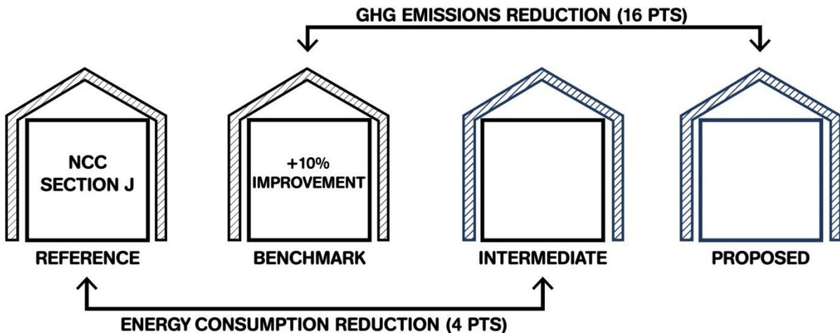
Figure 1: For *Green Star - Design & As Built* projects, the distribution of points based on the Reference, Benchmark, Intermediate and Proposed models.
