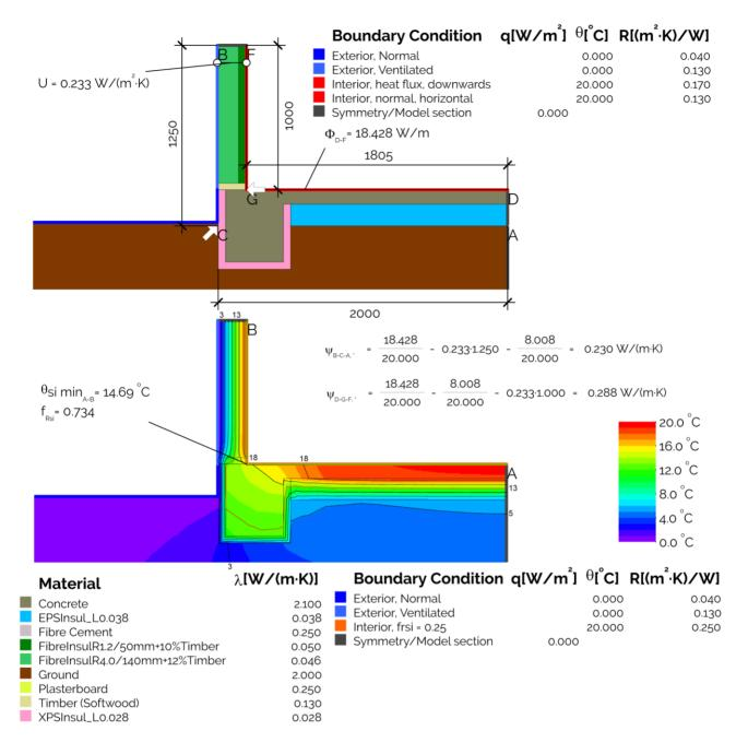
These CHI values have been calculated using a 3D finite element model, using ISO10211:2007, for a section of the slab edge A/P=2m with and without the timber pile.
