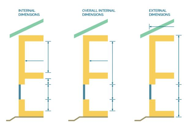
Figure 12: Area of the thermal envelope is measured using one of the following three systems normally used for component dimensioning: internal dimensions, internal overall dimensions or external dimensions. NZBC uses internal or internal overall depending on the project. The area is largest when using external areas and this area measurement is required for use in PHPP and the NZGBC V5 ECCHO tool based on PHPP. Illustration based on Berggren et al 2018.
