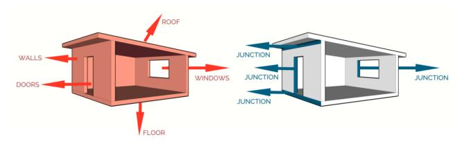
Figure 2: Elements (left) vs Junctions. High-performance buildings require Junction performance for sufficiently accurate predictive thermal modelling.
