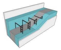
Detailed view of ICF showing the concrete and steel core with the plastic connectors holding the two sides of the blocks together; plaster outside and gypsum or plaster inside. Some ICF systems supply specialist foundations, midfloor and roof blocks.
