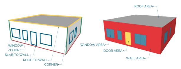
Figure 15: Example simple building with areas and junctions highlighted. Roof-to-wall length is shown in yellow; corner length in green; slab-to-wall length in red; and window/door-to-wall install length in blue.
