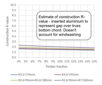
This graph of construction R-value assumes that the area over the truss bottom chords is an open-air gap to the ventilated attic and any heat entering this gap will quickly rise up and out of the building by air convection. Carefully fitting insulation around the truss webs to prevent gaps or using loose fill insulation is recommended.
