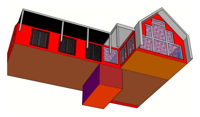
Figure 16: An example of a complicated building with an underground carpark, which has many thermal bridges Junctions. Even with good practice, they add significantly to the heat transfer.
