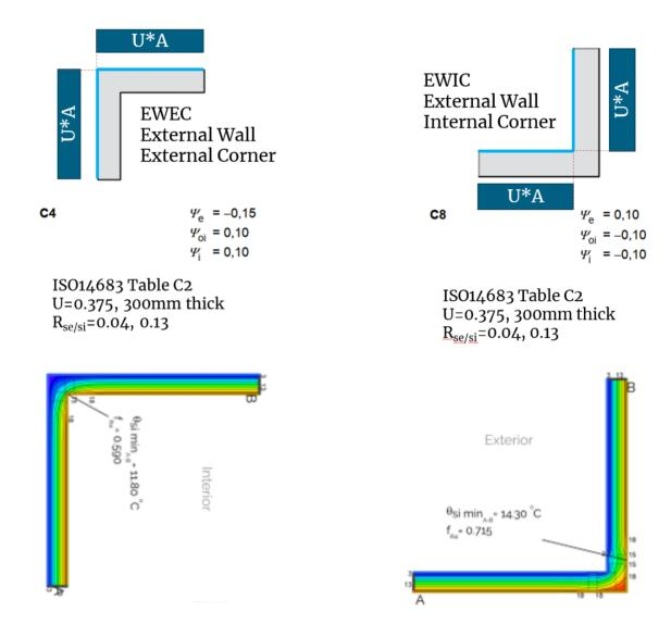
Figure 13: Thermal bridge values for corners and dimension systems.
