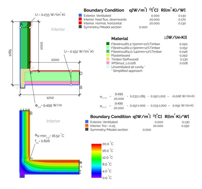
The boundary condition below the suspended timber floor would change depending on the subfloor void ventilation etc. The variation in the thermal bridge PSI value at the floor slab edge is small and the values provided here can be used for all cases while being only slightly conservative.
