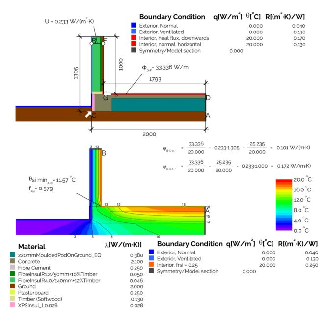
In the2D thermal bridge calculation, the 220mm tall waffle pod EPS foam with air pockets and concrete ribs have been replaced with an equivalent thermal conductivity calculated with a 3D finite element model using ISO10211:2007. Note that 100mm concrete ribs at 1200mm centres in the field of the slab have been assumed. The 300mm wide concrete edge beam is modelled as concrete as shown.
