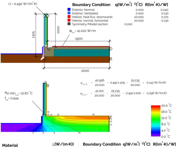
220mmMouldedPodOnGround\_EQ Concrete FibreInsulR2.2/90mm+12%Timber Ground Plasterboard Timber (Softwood) XPSInsul\_L0.028
