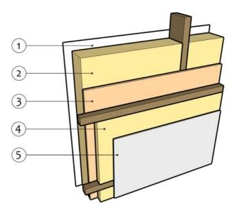
Figure 6: Element showing (4) 45mm service cavity to the inside of the rigid AVCL (plywood in this image).
