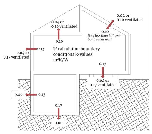
Figure 19: Air film surface resistances using ISO6946:2007. These were used for all Elements and Junctions. They differ only slightly from the NZS standard values.
