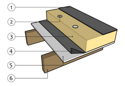
Membrane on rigid insulation warm roof:
