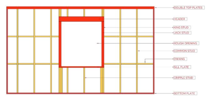
Figure 8: Timber to count with a 140mm tall timber lintel - accounted for in the thermal bridge of the window head.
