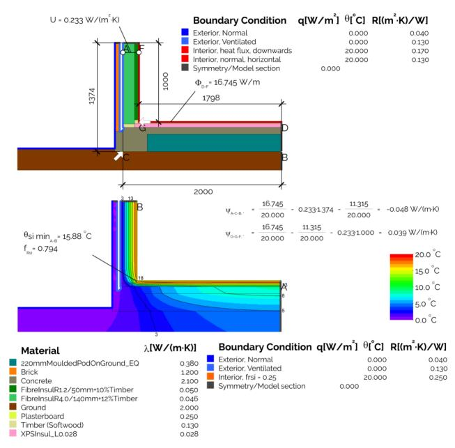
In the2D thermal bridge calculation, the 220mm tall waffle pod EPS foam with air pockets and concrete ribs have been replaced with an equivalent thermal conductivity calculated with a 3D finite element model using ISO10211:2007. Note that 100mm concrete ribs at 1200mm centres in the field of the slab have been assumed. The 300mm wide concrete edge beam is modelled as concrete as shown.
