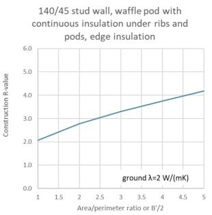
The insulated slab has the same materials and geometry as Junction 39. XPS ( $\lambda$ =0.028 W/(mK)) insulation 50mm thick on the edge and under the entire core of the slab with 220mm moulded pocket pods with 100mm concrete ribs at 1200mm centres on top of the XPS. Floor covering neglected.
