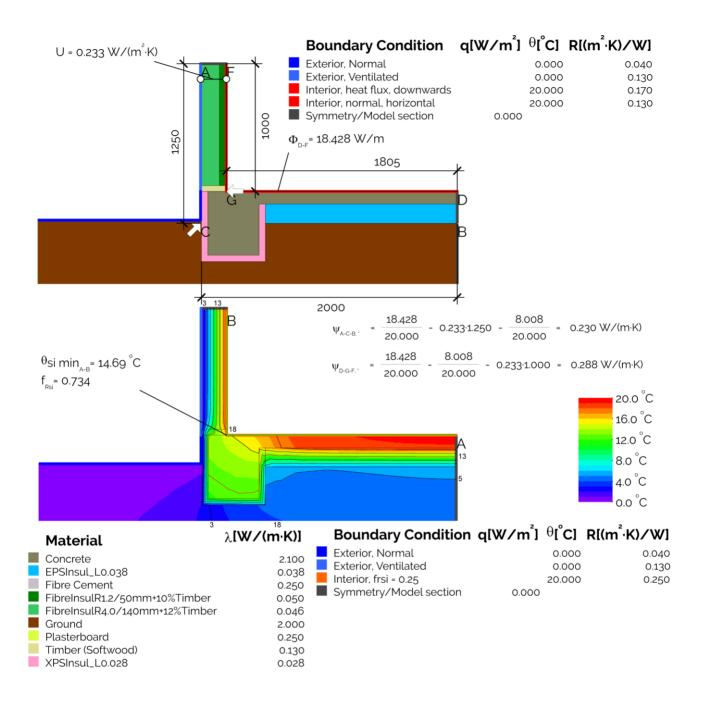
These CHI values have been calculated using a 3D finite element model, using ISO10211:2007, for a section of the slab edge A/P=2m with and without the concrete pile.
