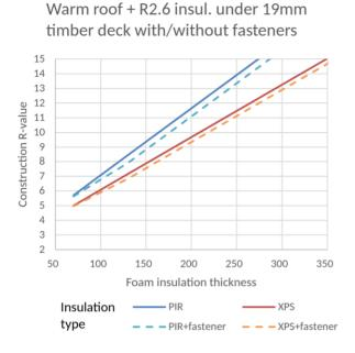
Fastener impact on thermal performance is calculated using ISO6946:2007 Annex D. Full thickness (non-countersunk) fasteners should be avoided. Countersunk fasteners have an impact on overall performance but are recommended along with fully adhered systems. Graph assumes 3.5 fasteners per sqm and 6.3mm steel screw countersunk 60mm , and then the countersunk depth increased so the steel screw is a maximum of 100mm long.
