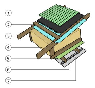
Figure 7: Element showing (6) timber blocking and metal batten system forming a ceiling service cavity.
