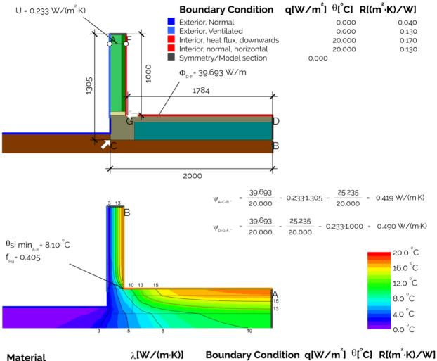
220mmMouldedPodOnGround\_EQ Concrete FibreInsulR1.2/50mm+10%Timber FibreInsulR4.0/140mm+12%Timber Ground Plasterboard Timber (Softwood)
