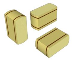
Note that the heat flow along the straw strands is higher than across them. This means the bales are more insulating when placed on-edge compared to flat, even though the bale laid flat is thicker. This is called anisotropic heat flow and is the reason that the different thermal conductivity values are used in the Element calculations. The common bale size is 900 mm long x 450 mm wide x 350 mm high (when placed flat). This means that the bales on edge are 350mm thick and on flat are 450mm thick.
