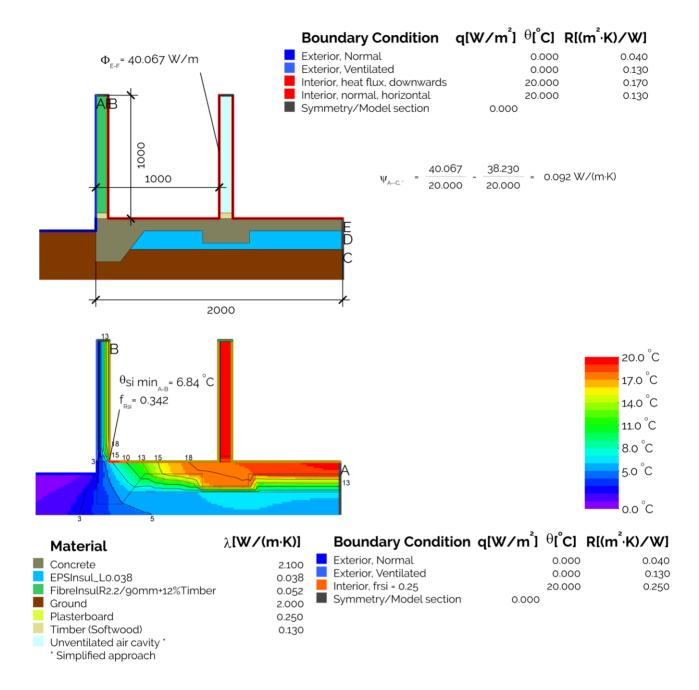
Calculating the thermal bridge impacts of slab thickening or other reductions in floor insulation at interior load bearing walls is conservatively estimated by calculation of the floor slab edge with and without the thermal bridge and subtracting. PHI has determined that a distance of 1m from the slab edge for a 2D thermal calculation is sufficiently conservative and significantly reduces the complexity of a 3D calculation.
