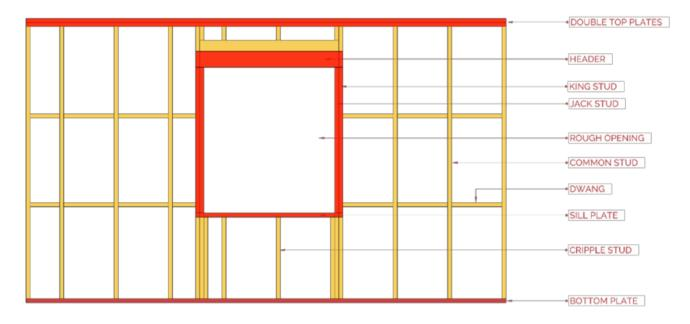
Figure 9: Timber to count with a 240mm tall timber lintel. This additional timber beyond 140mm needs to be added to the wall timber fraction.
