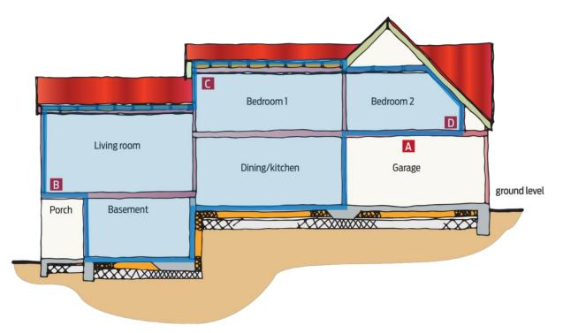
Figure 11: The thermal envelope is the surface between conditioned and unconditioned space. Illustration from *Build 159 34 Design Right Thermal Envelope Basics*.
