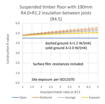
Analysis used a timber content in the floor at 12%. Floor R-value excludes the finish flooring but includes 20mm of wood board [ $\lambda$ =0.13 W/(mK)].
